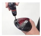
Adjust the weight with the sole surface oriented upward. The weight becomes movable after loosening the screw about two revolutions. However, the screw will come out if loosened too far.
